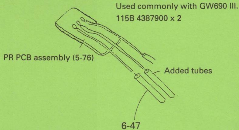
The tubes are added to prevent short-circuit.
