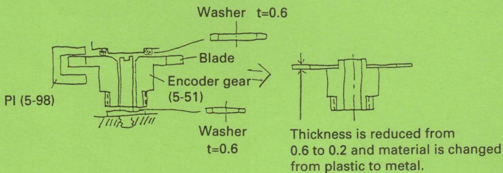
To provide more space in between the PI and encoder gear blade.
