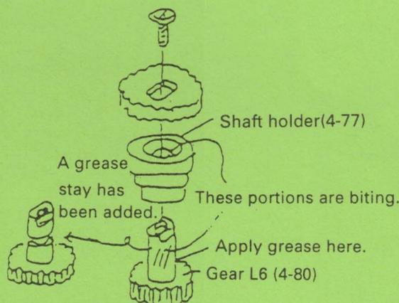
When this trouble is anticipated, replace the gear train assembly (4-55) with a new one. Do not replace the gear L6 (4-80) alone. The shaft holder (4-77) may have been worn.
