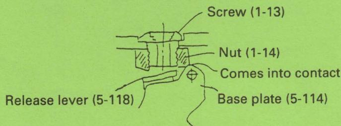
This change provides a space in between the nut and base plate.
