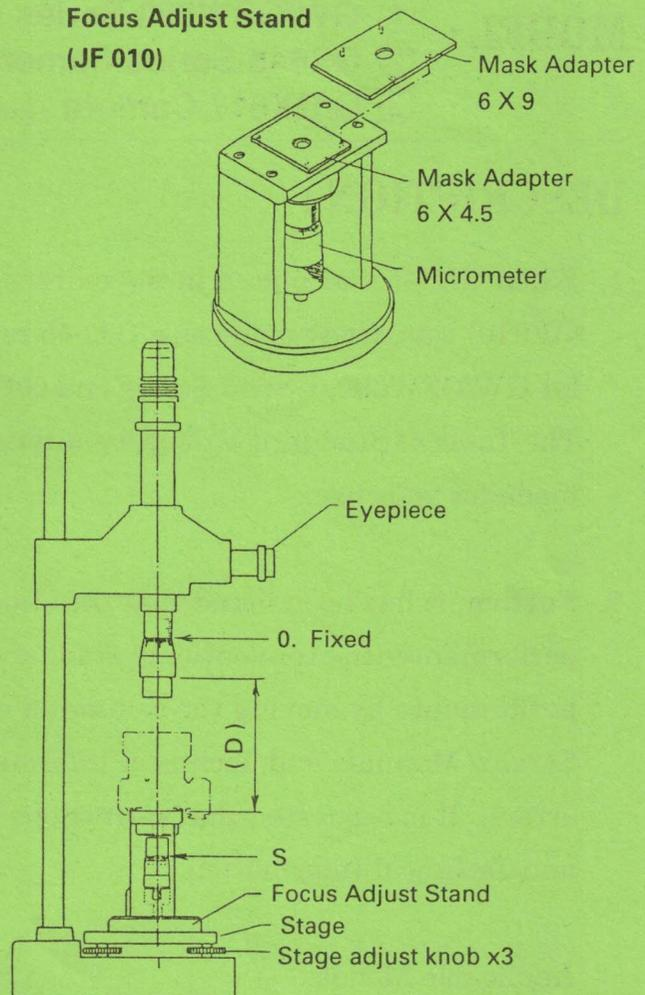
Note 1: Match the collimator objective lens scale accurately with the zero (infinity) position, correctly adjust diopter of the eyepiece, and adjust the collimator stage so that the stage is in right angle against the optical axis before starting to adjust focusing performance.
