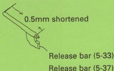
To secure function of the release bar.
